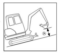
When travelling downhill, let the bucket slide along the ground, if this is possible on the type of ground in question.
