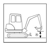
Push the two travelling joysticks (C-D) forward at the same time, the excavator will move straight forward. When these controls are released, the excavator will stop immediately.
