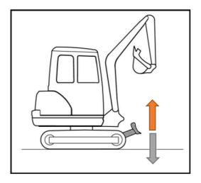
To move the blade down, push the joystick (B) forward.
